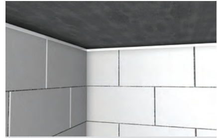
Top of wall construction joint
