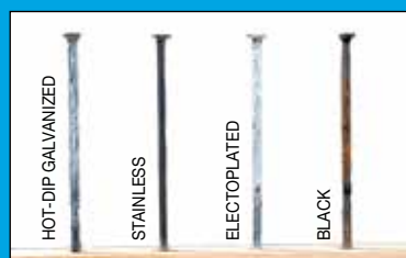
Nail samples after 96 hours (4 cycles) in the humidity chamber
