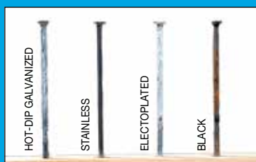
Nail samples after 24 hours (1 cycle) in the humidity chamber
