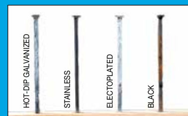
Nail samples after 168 hours (7 cycles) in the humidity chamber
